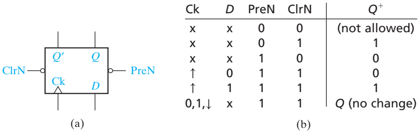
FIGURE 11-29 D Flip-Flop with Clear and Preset © Cengage Learning 2014
