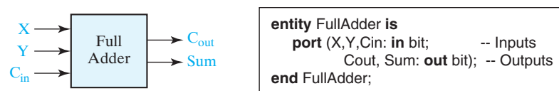
FIGURE 10-10 Entity Declaration for a Full Adder Module
