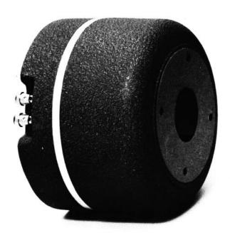
Model 2482 is an extremely high-power professional-quality compression driver. It has a 100 mm (4 in) voice coil and a magnetic structure weighing 10.5 kg (23 lb). It can take the most explosive transients in stride and reproduce them at thunderous levels. Model 2482 is built to typical JBL standards of precision.
