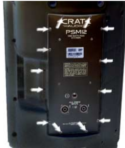
Figure 1: Remove the jackplate screws:
