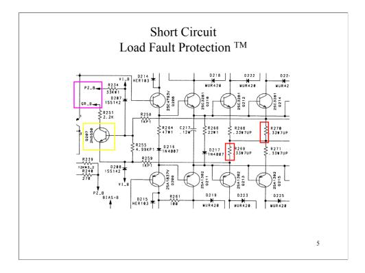
**GR\_B** is normally about +25 volts. Excessive current through R269 or R270 will indicate a load fault or short. **PZ\_B** is feedback from the output. If there is an output voltage (load fault condition) the voltage from **PZ\_B** will prevent Q207 from turning fully on. In this case **GR\_B** would reduce the input. Under a short, Q207 would turn on and the amp will enter the protect mode. This happens through SH\_B and PROT\_B not shown here.
