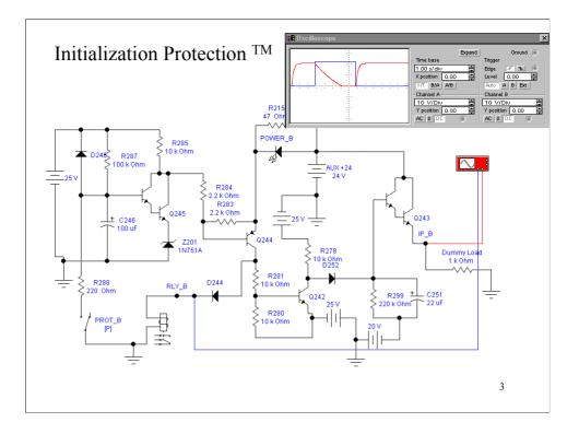
When power is applied to the GPS3500, RL200 isolates the amplifier from the speakers. Initially, Q245 has zero volts between the base emitter and will be off. Since Q245 is off Q244 will be off and RLY\_B will be low. While RLY\_B is low the RL200 will be off.
