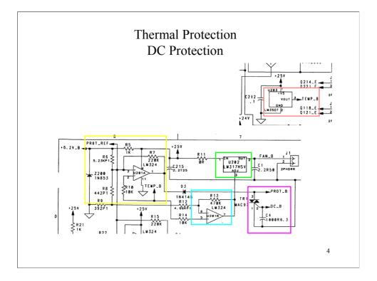
U203 is a precision centigrade temperature sensor. It's output will be 10mv for each degree centigrade. U202 is a three terminal voltage regulator. It's output is 1.25 volts higher than the voltage on the ADJ pin. U202 directly controls the speed of the fan. The TEMP B signal is applied to U201B which controls the fan speed through U202. R13 provides hysteresis. The fan will stop at a lower temperature than it started.
