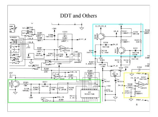
If the frequency and peak voltage of SH\_B cause C261 to charge up to greater than 6.2 volts then PROT\_B will go low an the amp will go into protect mode. Initialization will start over if that condition is removed. SH\_B originates from Q240 which is controlled by GR\_B (short and load fault) and Q241 which detects clipping.
