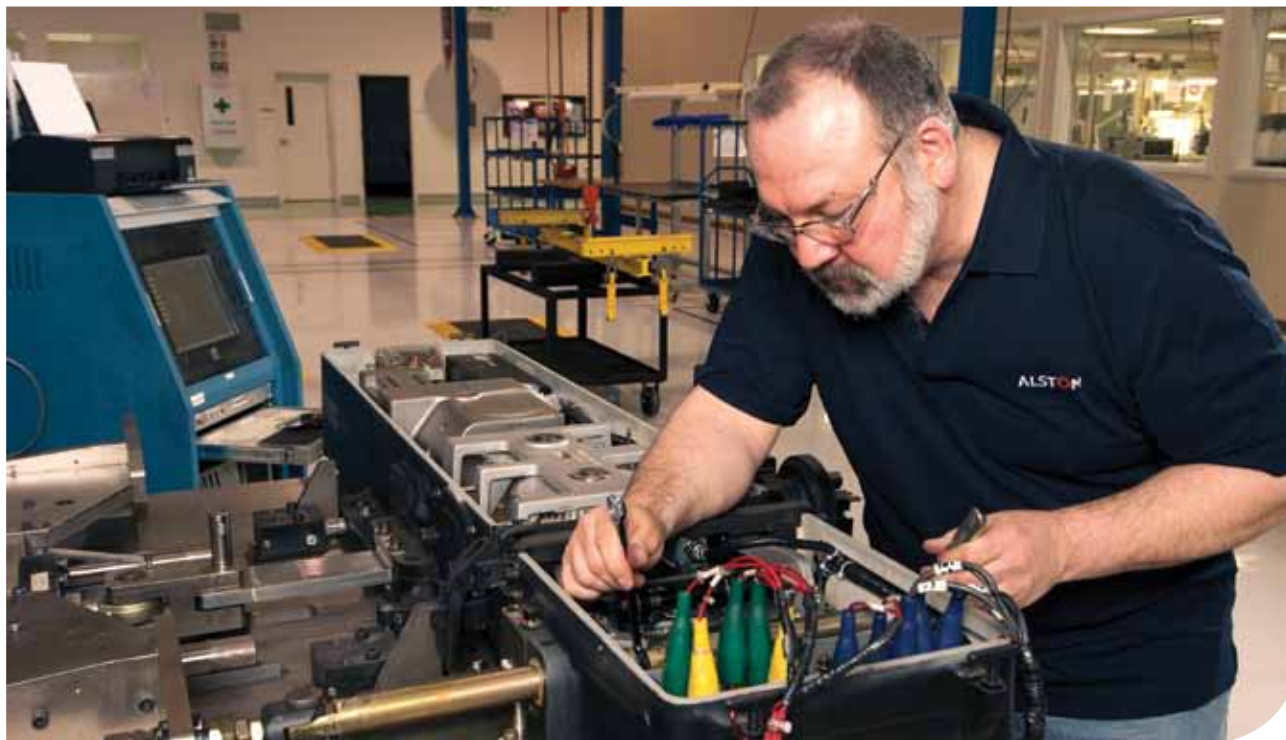
GM4000A™ Switch Machine being tested at the Rochester, NY facility
