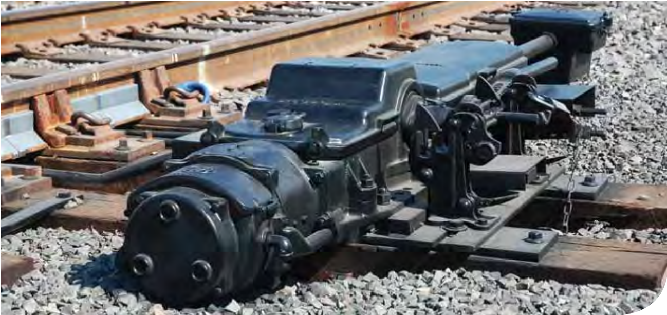
Model 5H Switch Machine installed at customer location
