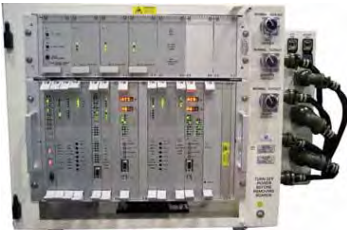
Micro Cabmatic™ III - OBC with full ATC/ACES functionality
