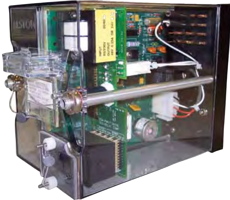
Microchron II Vital Timer Relay (AC)
