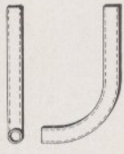
To be made from old boiler tube cut and bent as shown.
