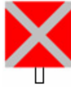
CROSSING WARNING DEVICE MALFUNCTION
