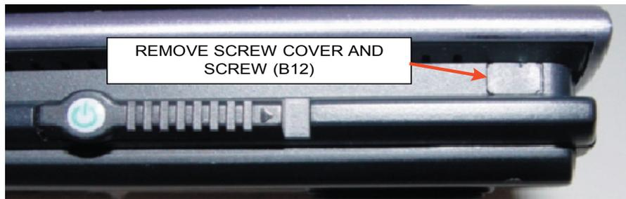
FIGURE 2-4 - SCREW COVER AND REATINING SCREW
