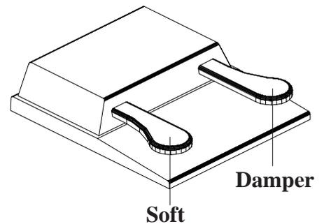
**Important:** Before using the pedals, make sure that the pedal cable is correctly inserted in the appropriate socket (**PEDAL SWITCH**) at the back of the instrument. If you want to use a single pedal, insert the jack into the **DAMPER** socket.
