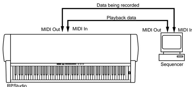
• **Important user info on MIDI cables:** always use high quality MIDI cables for your MIDI connections and avoid using cables longer than approx. 15 feet: cables which exceed this length tend to pick up unwanted noises and can cause data errors.
