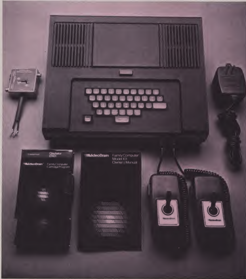
VideoBrain comes with keyboard console, two plug-in joysticks, AC adapter, TV-antenna switchbox, and several program cartridges.
