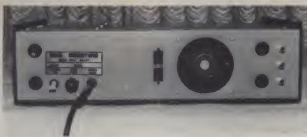
Interfacing the IIP is quite simple. The three RCA phono jacks on the back are for video out, tape in and tape out. The computer is also supplied with a fan to keep the innards cool.
