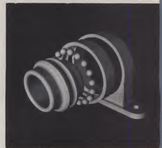
In this series of photos you see first a complete ball-bearing assembly, then the assembly with a box subtracted from one section to create a cross-sectional view, then the components separated to create an "exploded" view.
