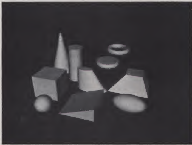
Pictured here are ten primitives used as building blocks in the SynthaVision process. From left to right they are: sphere, box, cone, cylinder, wedge, elliptical cone, solid torus, torus, arbitrary polyhedron, and ellipsoid.
