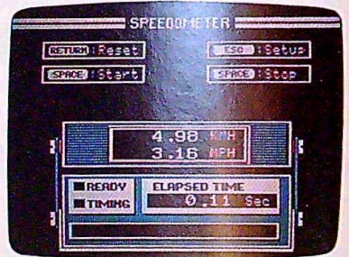
The Speed and Motion module turns an Apple II into a speedometer (shown here) and a tachometer.
