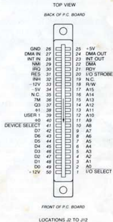
Figure 1. Peripheral Connector Pinout
