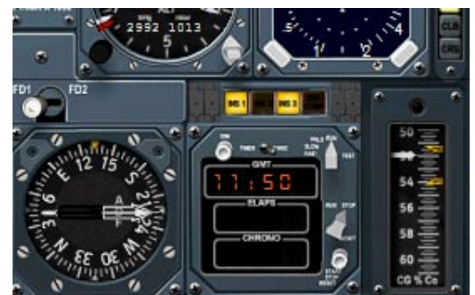
INS alert lights on the main panel
