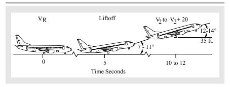
Retract the landing gear after a positive rate of climb is indicated on the altimeter. Retract flaps in accordance with the technique described in this chapter.
